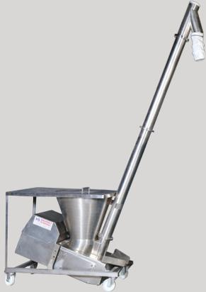
Screw Conveyor with hopper
